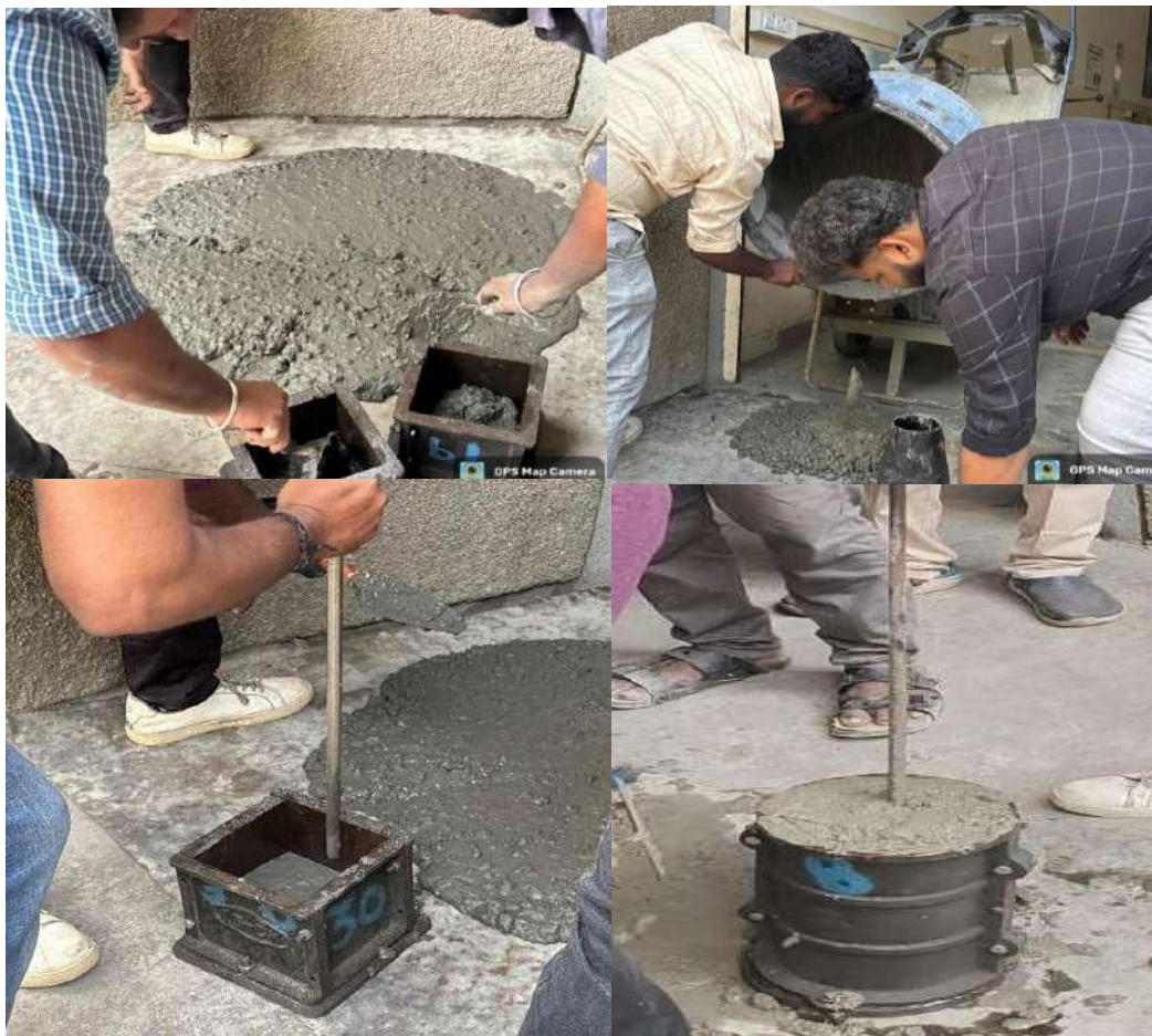
Fig 5.2 Casting of Specimens
