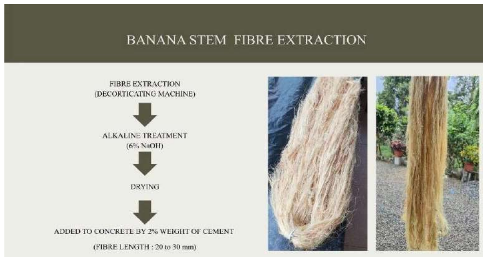
Figure 3.1: Making process of banana stem fibre
