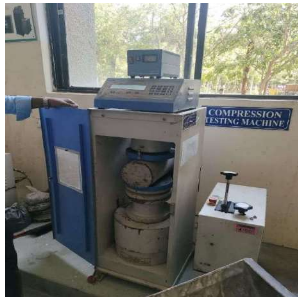
Figure 6.4: Conducting split tensile test
