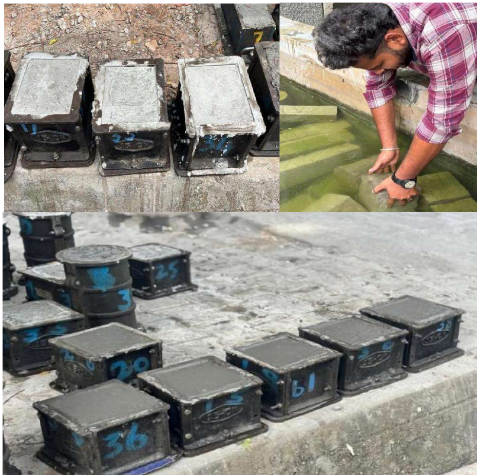
Fig 5.3 Demoulding and Curing
