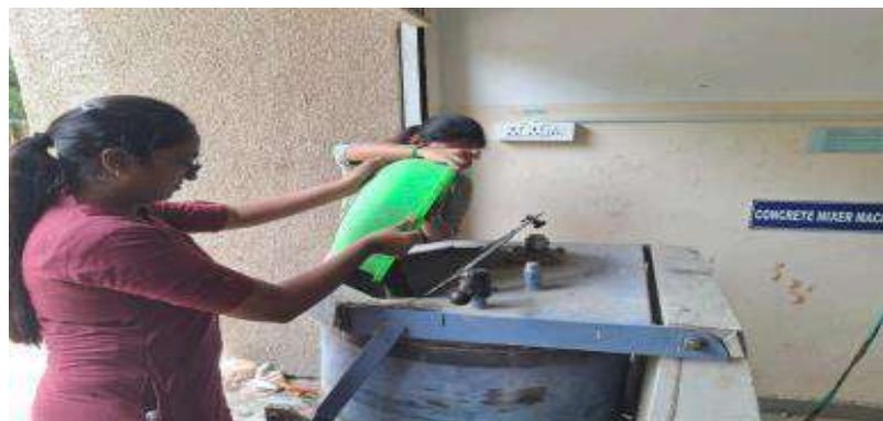
Fig 4.2. Mixture of concrete through Mechanical mixer
