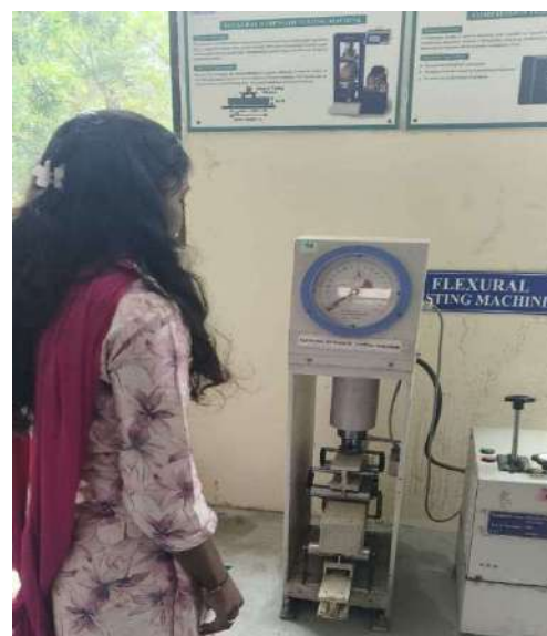
Figure 6.6 : Conducting flexural strength test
